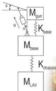
Underactuated control permits effective control of flexible light weight structures such as stabilized gun mounts
