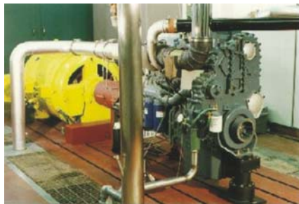
ORI's High Temperature Pressure Sensor Has Been Tested in a DDC Series 60 Diesel Engine at the University of Michigan Automotive Research Center.
