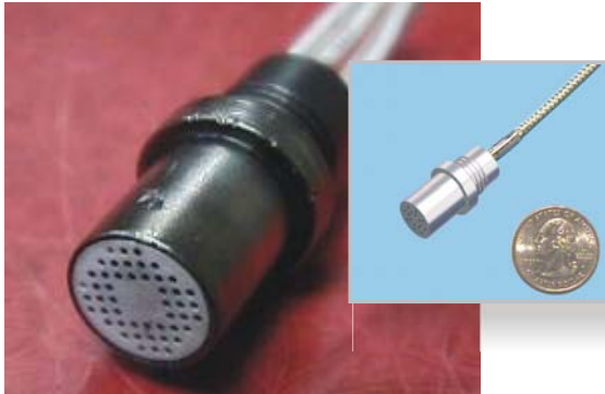
Packaged pressure sensor that flush mounts inside the combustion chamber.
