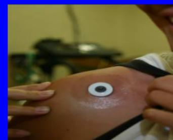
Figure 2. Dry Electrode in place on the skin
