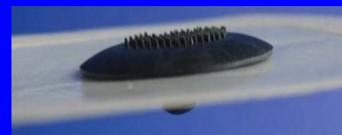
Figure 1 Photo Graph of the Novel Dry Electrode
