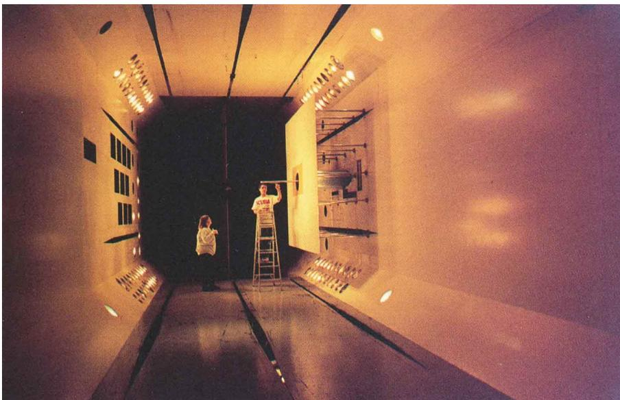
*Wind tunnel testing of ORICA intelligent control software has shown it to be highly responsive in damping out wing flutter. Application to commercial aircraft could result in safer and more cost-effective jet travel.*
